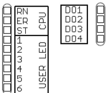
9 LEDs returns a feedback about input, output, software and hardware states.
