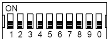
The DIP switches are in use to configure the CAN ID and bus termination, as well as the Ethernet IP address setting, if required.
