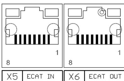
The EtherCAT bus from the PLC (= master) has to be daisy chained to X5 (= EtherCAT In) and X6 (= EtherCAT Out).
