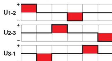
Figure 6-47 Block commutation of EC (BLDC) motors – Definition of phases
